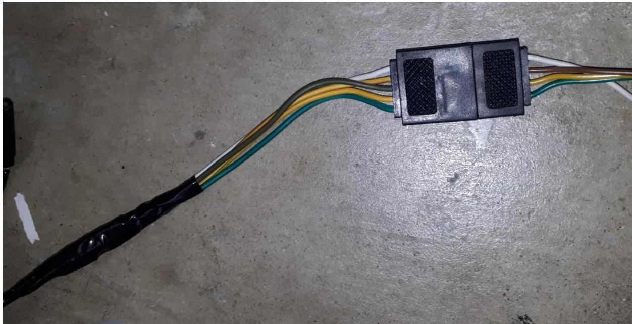
I put both units back in the panel, plugged them together and they worked like a charm. The flat 4 connectors don't have marine grade wire but it is pretty dry behind the dash. I am confident that it will be OK. During final installation, I sealed the joint between the two parts with electrical tape.
