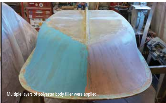
The old cracking gelcoat was stripped from the boat and multiple layers of fibreglass cloth and resin were applied.
