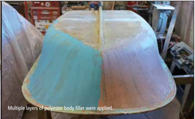
The old cracking gelcoat was stripped from the boat and multiple layers of fibreglass cloth and resin were applied.
