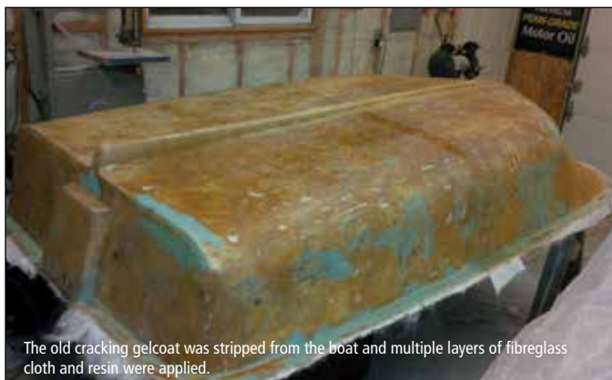
Multiple layers of polyester body filler were applied..
