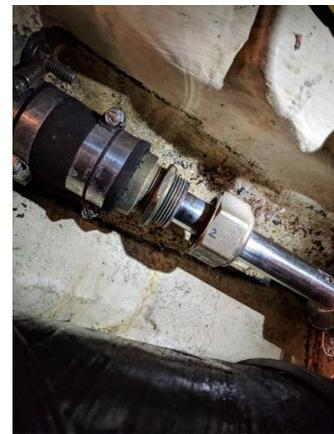
Repeat with the second wrap of packing. Set the packing material joint 2 nut faces (120 degrees) from the first. Mark the nut to show where the joint is.
