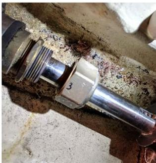
With all three wraps of packing pushed into the nut, hand tighten the nut to close the stuffing box. Tighten the lock nut to ensure the nut doesn't unwind when the engine is in drive.
