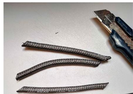
The packing material is selected based on the size of the stuffing box. With Vernier calipers, measure the diameter of the drive shaft and the internal diameter of the stuffing box nut. Subtract the shaft diameter from the internal diameter of the nut and divide by 2 to find the thickness of the packing material required. Order enough packing material to go around the shaft about 4 times.
