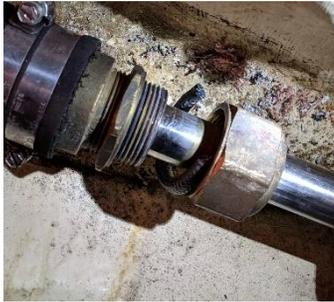
Since the drive shaft on my boat is 1" diameter, I used a spare piece of SS 1" tubing to wrap the packing and measure the lengths for cutting. This is easier than trying to do the measurements and cutting on the actual shaft. The best way to cut the packing is a mitre cut at 45 degrees with a razor knife. This allows the packing to compress tighter and allow less water to flow into the boat. The cuts are made to leave a tight fit around the shaft.
