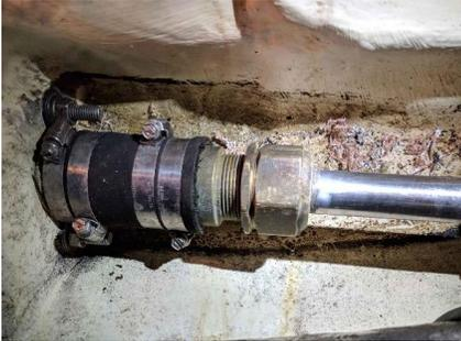
Boats with inboard engines where the drive shaft goes through the hull to turn the prop need some method to prevent water from entering the boat through the drive shaft opening. For over a hundred years a simple method called a stuffing box has been used and is still found on most inboard engine boats. Some boats have a dripless shaft which uses a complex mechanical device to keep water out.
